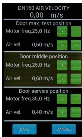
The device is equipped with an air velocity measuring and control system.
